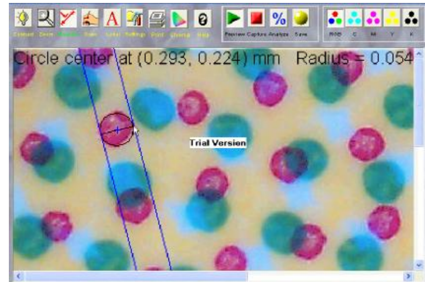
Measurement of a printing dot With numerical information for diameter, distance, length and so on!
